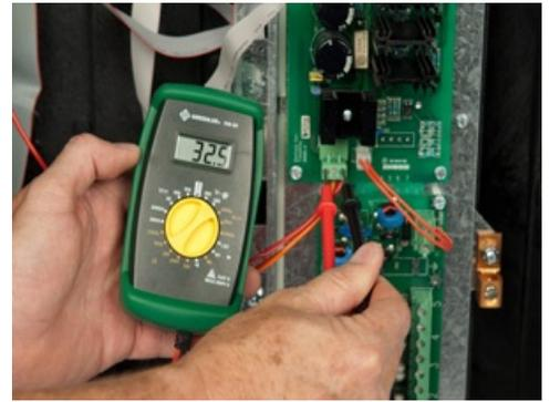
3. Next, put the same testing probes on a pair of Decoder Wire Path terminals (flat head screws) and see that voltage is making it's way through the Decoder Output Board. If there is a fluctuating voltage ranging from 22V to 80V then the Transmitter Board and Decoder Output Board are still in a working capacity.
