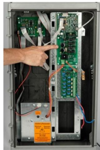
2. With a volt meter, put a single probe on each side (flat head screws) of the lower wire harness. The transformer feeds this board directly with a consistent 32V of AC current. Be sure that the Transmitter Board is receiving the necessary voltage from the transformer.
