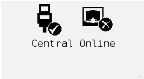
2. Field interface connectivity with the central computer is shown. Should both USB and ethernet cables be connected at the same time the system will use the ethernet connection.
