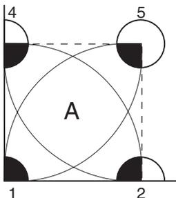
Sprinklers 1, 2, 4, and 5 are a quarter-circle head, two half-circle heads, and one full-circle head, respectively. The total GPM for the area is:
