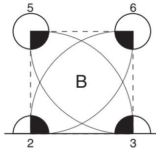
These are two half-circle heads with 2 GPM nozzles, and two full-circle heads with 4 GPM nozzles. The total GPM is:
