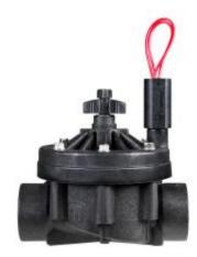
Brand: Residential & Commercial Irrigation Product Line: Valves Product Model: ICV SKU: ICV151G Description: ICV Valve, 1½" (40 mm) glass-filled nylon globe valve with flow control UPC-A: 0611698111871 Qty. / Bag: 8 Master Carton: 8 Land Pallet: 256 Ocean Pallet: 320 Feature Options: Flow control Inlet Size: 1½"
