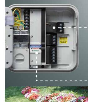
3-Station base controller expandable to 15 stations with PCM modules.
