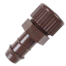
PLD-CAP 17 mm barb x 1/2" MPT with cap
