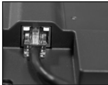
Network Lights (back of Com module)
