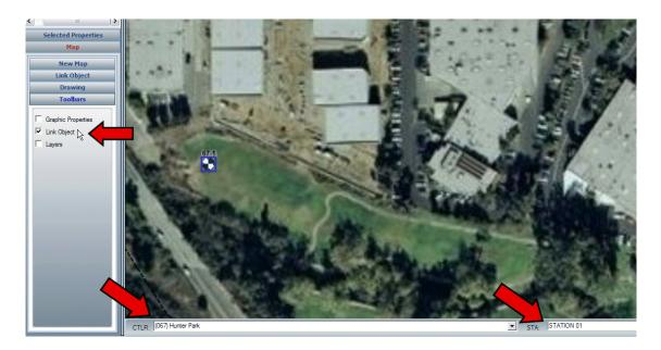
Select the linked object in the map that you want to change, and the link will be displayed in one or both of the fields at the bottom. You can use the down arrow next to these fields to change the link for the individual object.
