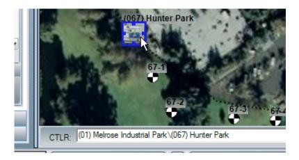
If the boundary for the controller has already been created and linked, this may be difficult or impossible without using the Layer tool. Sometimes the map will not let you place a controller symbol into the same area as the controller boundary.
