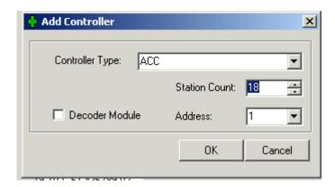
When the controller is configured for the correct number of stations, click OK.
