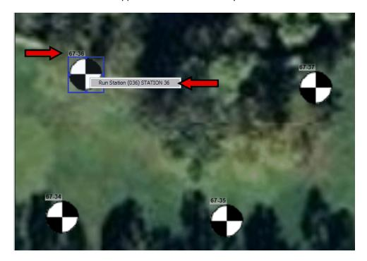
You can select, then right-click on any station in the map, to access the Run Station command for that station. Select Run Station and the Run Station dialog will appear. Enter the number of minutes for the station to run, and the command will be sent to the controller immediately.
