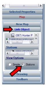
Select the Site, and expand to see the controller. Click the markers next to the Sites to expand the controllers, and click the controller for which you are placing stations. The stations will appear in the window.
