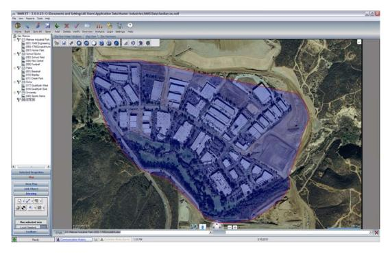
When you are finished, RIGHT-click to end the shape. The boundary will be complete, and will be automatically linked to the item (Site or Controller) you highlighted in the tree-view.
