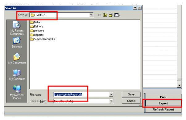
Not all delays reported in the Station Activity report are problems. If a station has Cycle and Soak settings, or Delay between Stations set for the program, the delays will be reported along with the run times. The Station Log in the controller records all activity, good or bad. Be sure to read the complete description of any reported event to fully understand it, before assuming that there is a problem.
