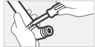
2. Tighten clamp around pipe and fitting.
