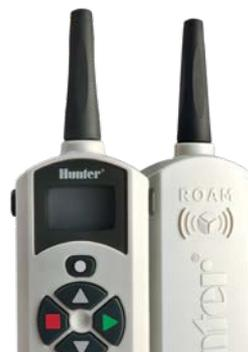
The Hunter ROAM Remote Control Kit saves time during installation and routine system maintenance. The receiver (right) plugs into the Controller Connection Kit and the transmitter (left) activates the sprinklers within a 300 m range. The user can manually run any zone without resetting the controller. Compatible with X-Core, X2, Pro-C, ICC2, and HPC controllers.
