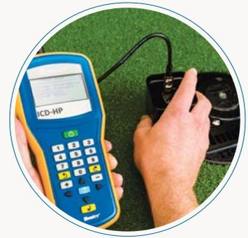
With the ICD-HP handheld programming and diagnostics tool, you can wirelessly program and interrogate every TWM from the surface. Communicate directly with TWMs and get digital confirmation of TWM functionality so you know wire paths are in working order.
