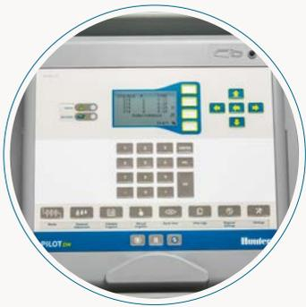
The control panel has a large, multi-language display with quick-access buttons for the most commonly used functions. Each hub can store and execute full watering instructions independent of the central computer.
