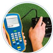
With the handheld ICD-HP Programmer, you can wirelessly program and interrogate every TWM from the surface. Communicate directly with TWMs and get digital confirmation of TWM functionality so you know wire paths are in working order.
