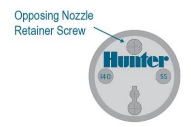
For opposing I-40 models, repeat steps 1 & 2. Install a smaller secondary nozzle on the opposite side of the rotor. For best nozzle selection, use the second nozzle performance charts in the spec section. <u>Learn More</u>
