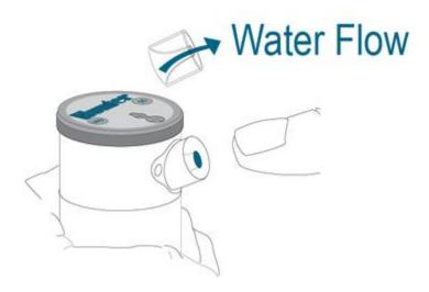
Discard nozzle if removed with pliers. Slip the desired nozzle into the nozzle socket. Note that the socket is angled up 25°. Tighten the nozzle-retainer/range-adjustment screw.
