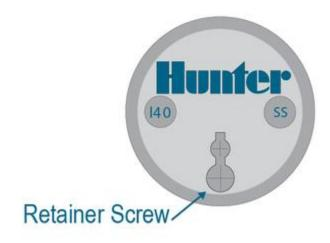
Using the Hunter wrench, loosen the nozzle-retainer/range-adjustment screw. If a nozzle is already installed in the sprinkler, it may now be removed by briefly turning on the water or removing it with pliers.
