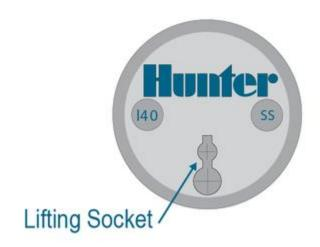
Insert the white key end of the <u>Hunter Adjustment Wrench</u> into the lifting socket of a pop-up sprinkler. Pull the riser up to gain access to the nozzle socket.
