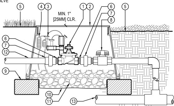
IN-LINE VALVE (IBV-151G) WITH ACCU-SYNC, UNIONS AND ISOLATION VALVE
