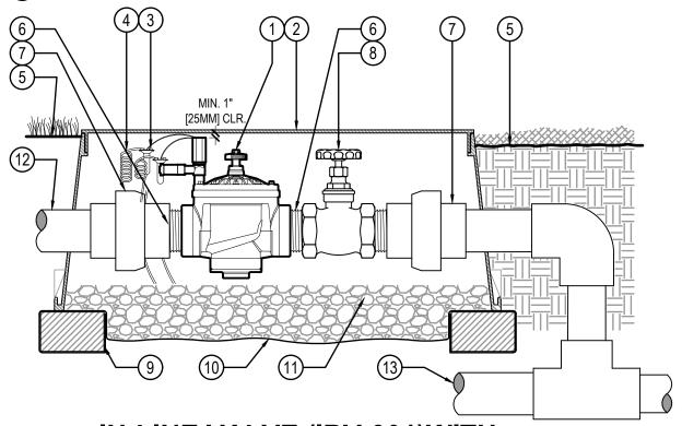
IN-LINE VALVE (IBV-301)WITH ACCU-SYNC, UNIONS AND ISOLATION VALVE
