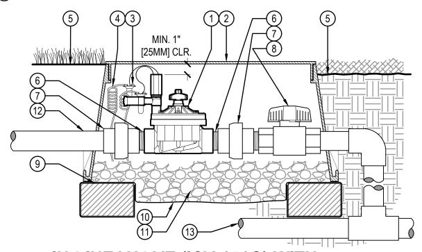
IN-LINE VALVE (ICV-151G) WITH ACCU-SYNC UNIONS AND ISOLATION VALVE
