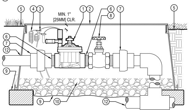
IN-LINE VALVE (ICV-201) WITH ACCU-SYNC, UNIONS AND ISOLATION VALVE
