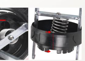
To remove the inlet valve, it is necessary to align the pointer arrow on the G900 Valve Tool with the alignment dot on the rotor's flange. The alignment dot is centered on the flange compartment lid adjacent to (next to) the body cavity opening. A second alignment dot is located below the lid in case the flange compartment lid has been removed. Align the pointer arrow on the tool with the alignment dot (FIGURE 94) and lower the tool into the rotor's body (FIGURE 95).
