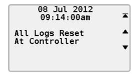
3. The log will show one entry at a time starting with the most recent. Use the UP ▲ and DOWN ▼ buttons to move to other log entries. The TOP ▲ button returns you to the most recent log entry.
