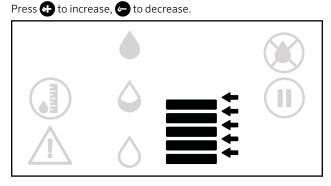
When the moisture level is reached, Soil-Clik stops the irrigation. This is shown by the  $\textcircled{\mbox{symbol}}$  symbol.
