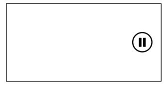
Pause does not pause watering. It overrides the Soil-Clik, and allows watering.
