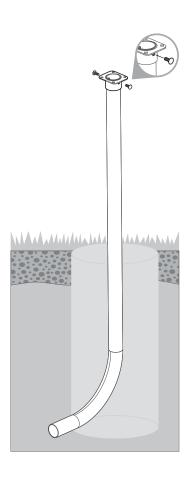
• Route all wires up the pole until at least 12" (30 cm) of wire extends out of the top.
