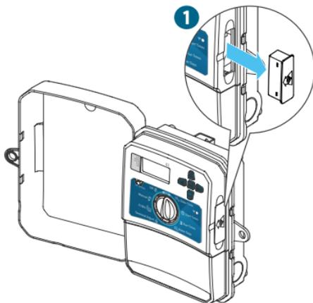
When installed, WAND disables the controller's dial and button functions, the existing schedule, and settings.
