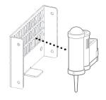
Attach the desired sensor without sensor arm to the screw bolt and securely fasten and reinstall enclosure screws.
