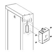
Attach the front plate of the guard and securely fasten with the provided screws.
