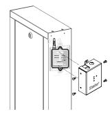
Attach the front plate of the guard and securely fasten with the provided screws.
