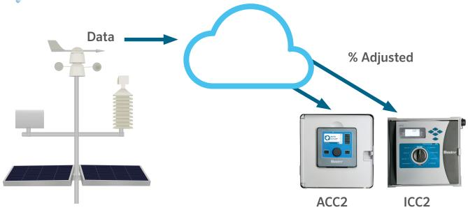
The alternative weather source can be used to calculate a percentage adjustment similar to that performed by the Solar Sync Sensor. It's also capable of adjusting all controllers to a specific percentage using the Seasonal Adjust commands. This is a simple formula based on the modified Penman-Monteith equation for evapotranspiration.
