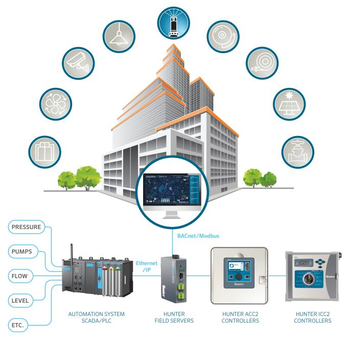
**Hunter commercial ACC2 and ICC2 Controllers** provide scalable, state-of-the-art irrigation control, leak detection, and water management when synchronised with your building management system, smart city, or wide-area SCADA applications. Multiprotocol gateways and drivers seamlessly integrate into BACnet<sup>®</sup>, Modbus<sup>®</sup>, and more than 120 other automation protocols.
