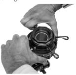
For 360° operation, remove both adjustment rings.
