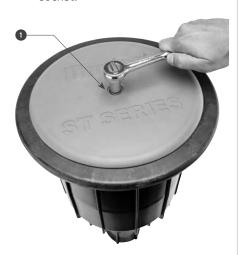
Use the gear-drive insertion/ removal tool to unscrew the rotor from the piston. The tool will grab onto the screws below the rotor.
