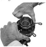
For 360° operation, remove both adjustment rings.
