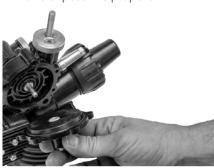
Remove the propeller from the housing to clear any debris that may be trapped inside.
