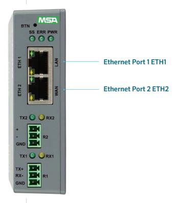
The Ethernet port is used both for BACnet/IP communications and for configuring the gateway via the Web App. To connect the gateway, either connect the PC to the router's Ethernet port or connect the router and PC to an Ethernet switch. Use Cat-5 cables for the connection. **NOTE:** The Default IP Address of the gateway is 192.168.2.101, and the Subnet Mask is 255.255.255.0.
