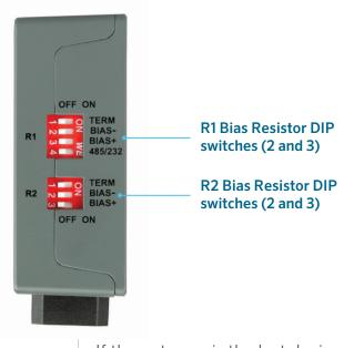
If the gateway is the last device on the serial trunk, then the End-Of-Line Termination Switch needs to be enabled. To enable the Termination Resistor, move the TERM dip switch to the right in the orientation shown above.
