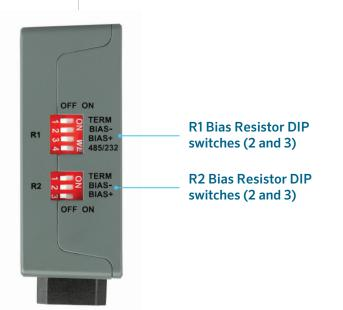
To enable Bias Resistors, move both the BIAS- and BIAS+ dip switches to the right in the orientation shown above.
