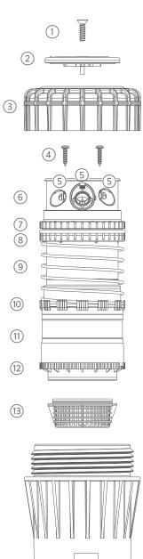
\*Parts 7–11 are required for the new I-90 seal replacement kit
